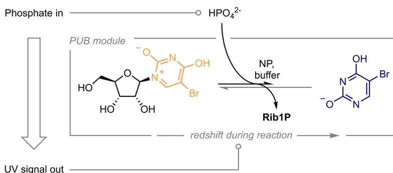
We herein introduce PUB, a module for phosphate detection by continuous UV-spectroscopic monitoring of 5-bromouridine phosphorolysis. The PUB module uses cheaply available, bench-stable reagents and can be employed for continuous and discontinuous reaction monitoring in biochemical assays to detect (pyro-)phosphate concentrations spanning almost 4 orders of magnitude, as demonstrated with representative use cases.
